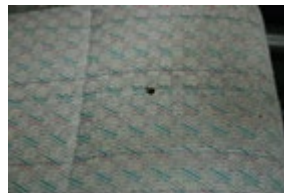
Brandgat in de stoelbekleding
