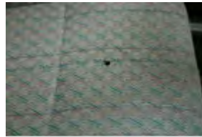
Brandgat in de stoelbekleding
